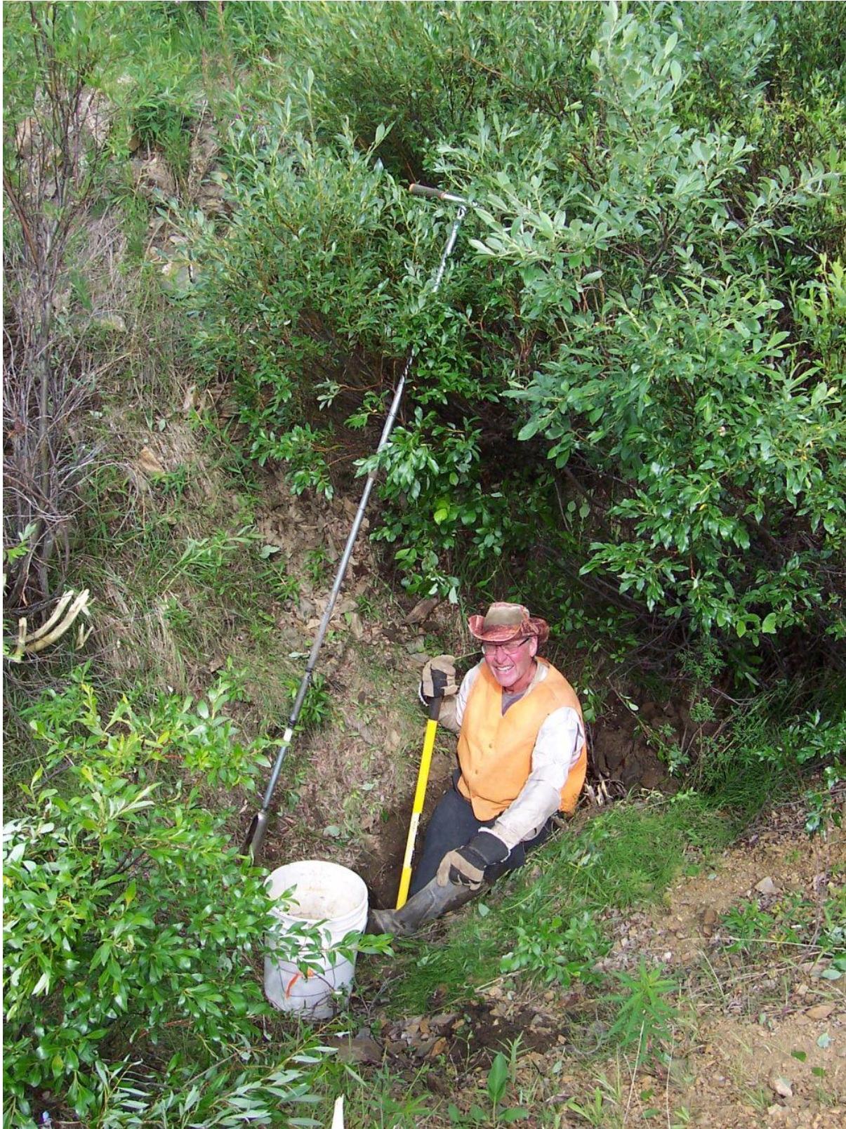
Photo 5. W. Hood digging pit to sample gravels below bottom of old excavator pit near east end of prospecting lease.
